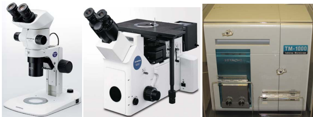
FIGURE 3 (left) Olympus SZX7 stereoscope (center) Olympus GX51 inverted microscope and (right) Hitachi TM-1000 tabletop SEM.
