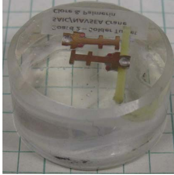
FIGURE 2 Polished sample holding two turret cross-sections.
