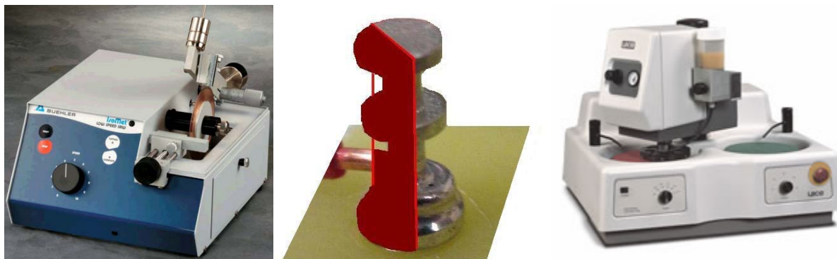
FIGURE 1 ( left ) Isomet low speed saw by Buehler. ( www.buehler.com ) ( center ) Area removed using Isomet saw. ( Right ) LECO Spectrum 1000 ( www.purdue.edu/mse )
